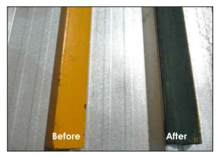
the container door with the first application of CM707; the layers of paint had softened and came off with the scraper in strips. It was necessary to make two more applications with the CM707 and to remove all the layers of paint from the container door.
