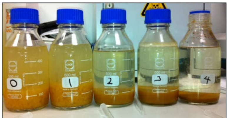
Example of wastewater from an oil production platform treated with a two-stage electrocoagulation system supplied by Global Advantech
