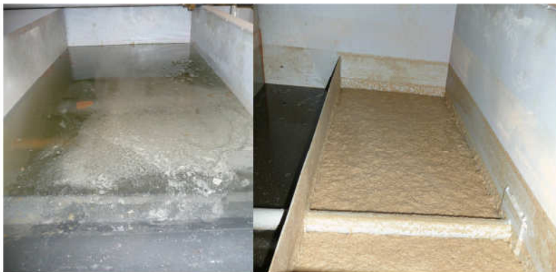
Gas bubble and floc production in flotation/sedimentation tank
