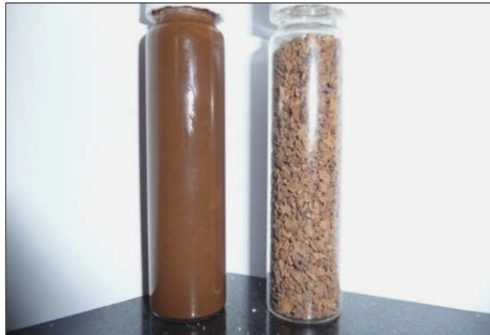
The resulting separation of larger particulates (right) from oil well drill cuttings ex BP Wytch Farm (left)
