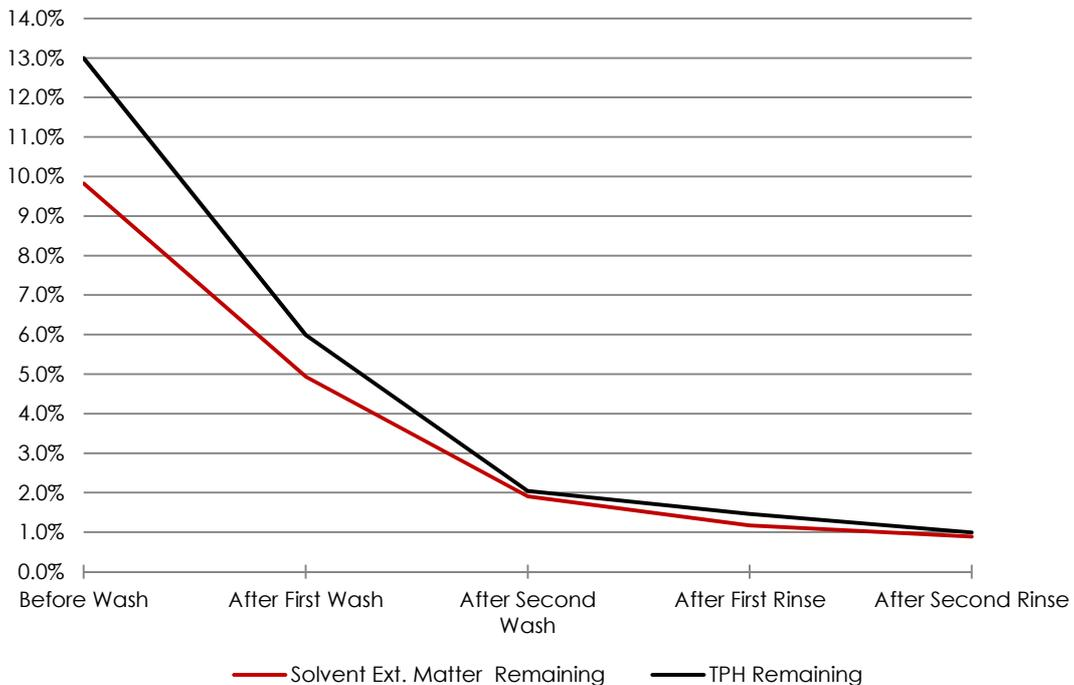
The crude oil remaining in the oil well drill cuttings during the full washing cycle: before the trial after each washing and rinsing stage.
